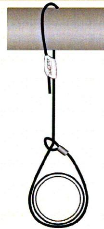
Single point cradle configuration with Gripple Fastener at the top.
