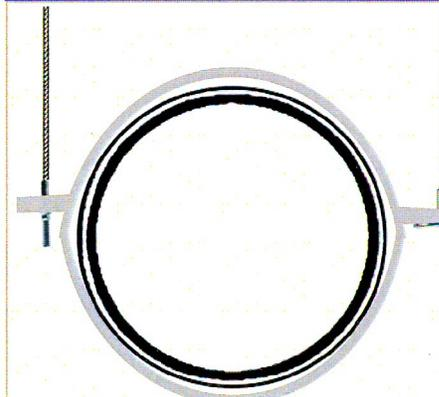
Where the spiral or round duct is supported with top & bottom bands, Gripple cable hangers are attached to the bands via a Stud end fixing (left) or 90° Eyelet end fixing (right).
